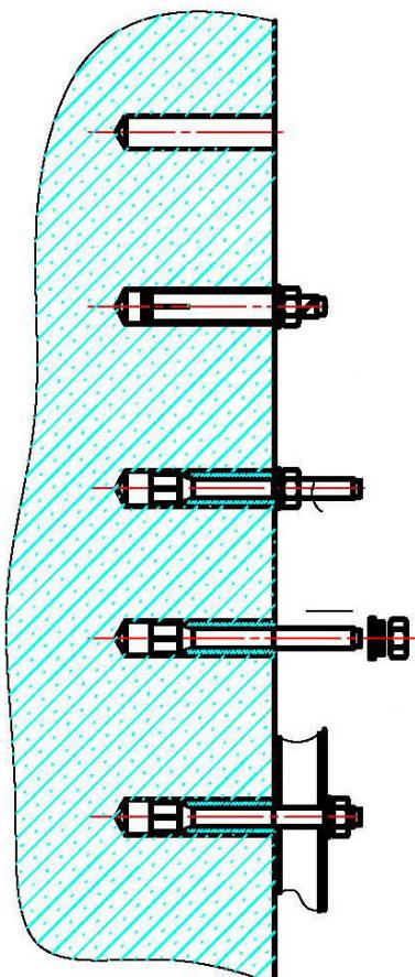
Punch a hole, no less than 60mm.
